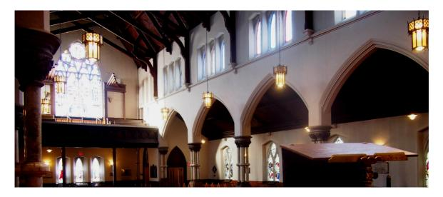
The great rafters and beams of the roof, the four-inch thick floor boards and the pews are all made of white pine, the wood that was the foundation of the region's economy for much of the 19th century, and into the 20th.
